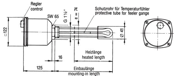
For pressure reservoirs made of refined steel or enamelled steel and anode screw-in type heaters ERCTBi will be used. In this finish the tubular heaters are mount galvanic isolated from gland G 1 1/2". Thereby, the protection current is prevented by the tubular heaters and the cathodic corrosion protection of the container barrier remains.
